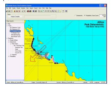
**Figure 5** Example SEATide prediction model interface for the Townsville region in North Queensland
