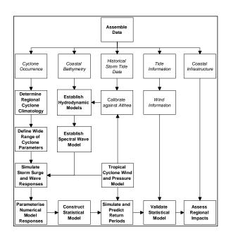
**Figure 1** Example coastal hazard study methodology.
